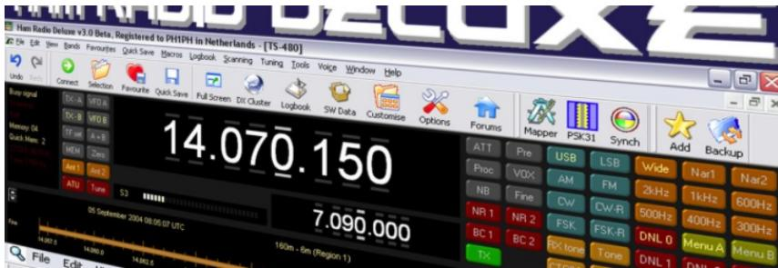
One of the first features you set up is CAT control PTT control so that your Digimode software can set and get the frequency and mode of your radio and make it transmit. First you need to ensure that you have the right driver installed.
