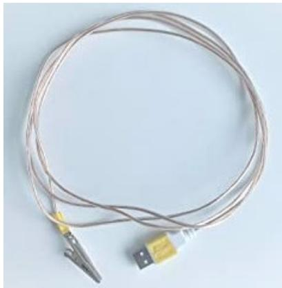
However, one option for grounding a laptop or PC is to use a USB Grounding lead. This will connect the screen/0v line of a USB Plug to a crocodile clip which you can attach to your station ground bar. Pop one of these into a spare USB port and then to your station earth and they can work wonders.
