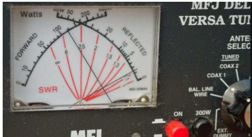
Before I get too deep into setting up transmit audio, there are some regular transmit problems that we see, the most common being no (or too low) output power. This could be due to the default sound card you have set in Windows or the radio not being in the correct mode to enable the audio input pin on the data port.
